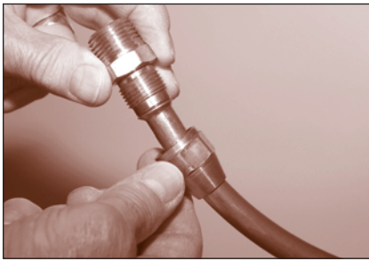
FIGURE 28: Flare fitting/flared joint during assembly
