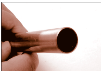
FIGURE 82: Prepared tube end
