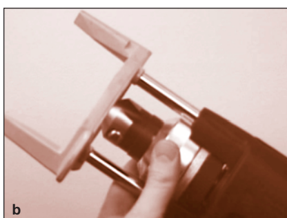
FIGURE 95 (a and b): Retracting the forming pins
