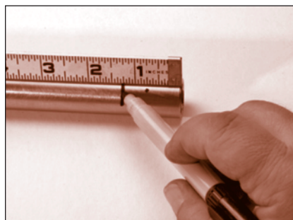
FIGURE 85: Marking insertion depth
