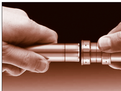
FIGURE 72: Aligning tube end squarely
