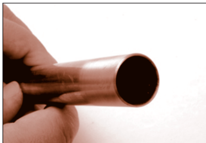
FIGURE 69: Chamfered tube end
