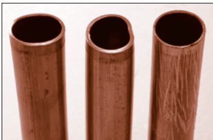
FIGURE 45: Inspect tube for imperfections
