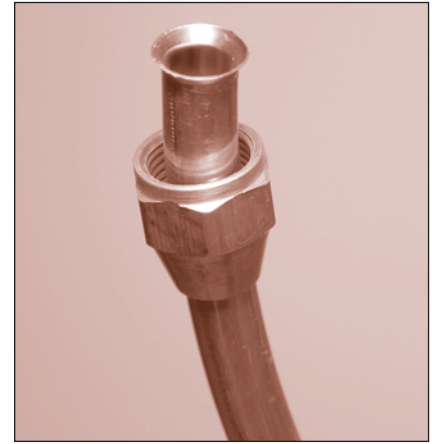
FIGURE 32: Completed flared tube end
