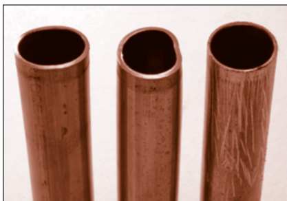
FIGURE 64: Ensure tube is clean, round and free of imperfections
