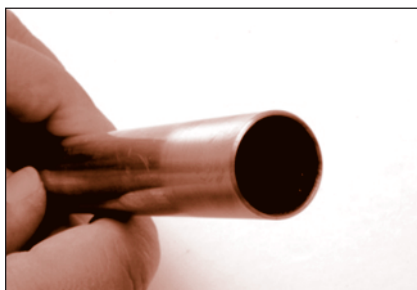
FIGURE 55: Properly prepared tube end
