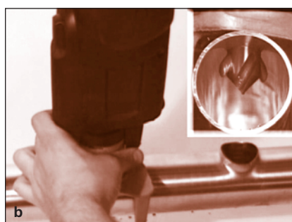
FIGURE 97 (a and b): Extending the forming pins inside the run tube
